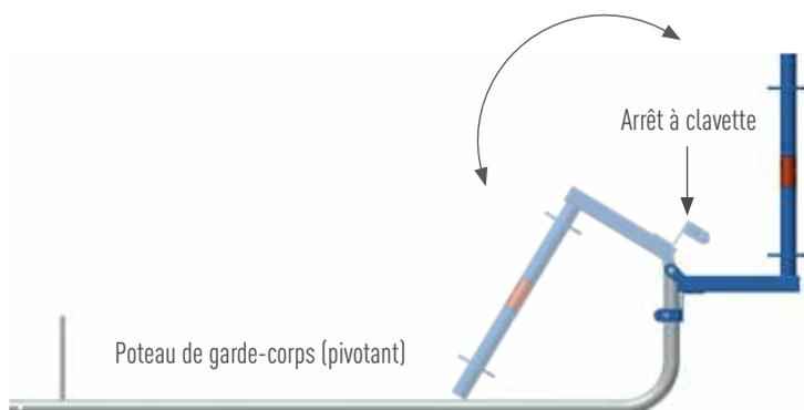
**AIDE À L'ASSEMBLAGE GARDE-CORPS TOIT PLAT**
