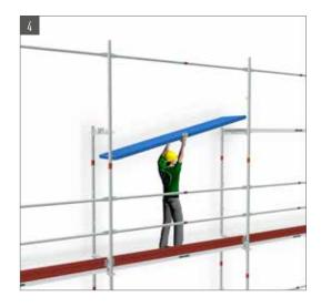
The scaffold decks are laid around the work complete this scaffold level.
