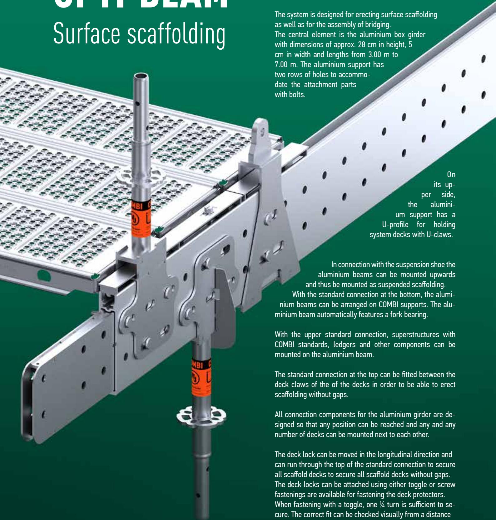
The MJ OPTI-BEAM support system is used together with components from the MJ COMBI system with U-support system decks.
