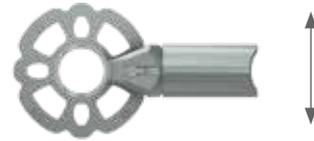
$V_{y,R,d} = \pm 17,3 \text{ kN}$
